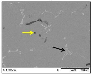
Fig 1: Microstructures of the 6351 aluminum alloy samples with different copper content; porosity (yellow marked); Al (MnCuFe) Si constituent (black marked) [18]
